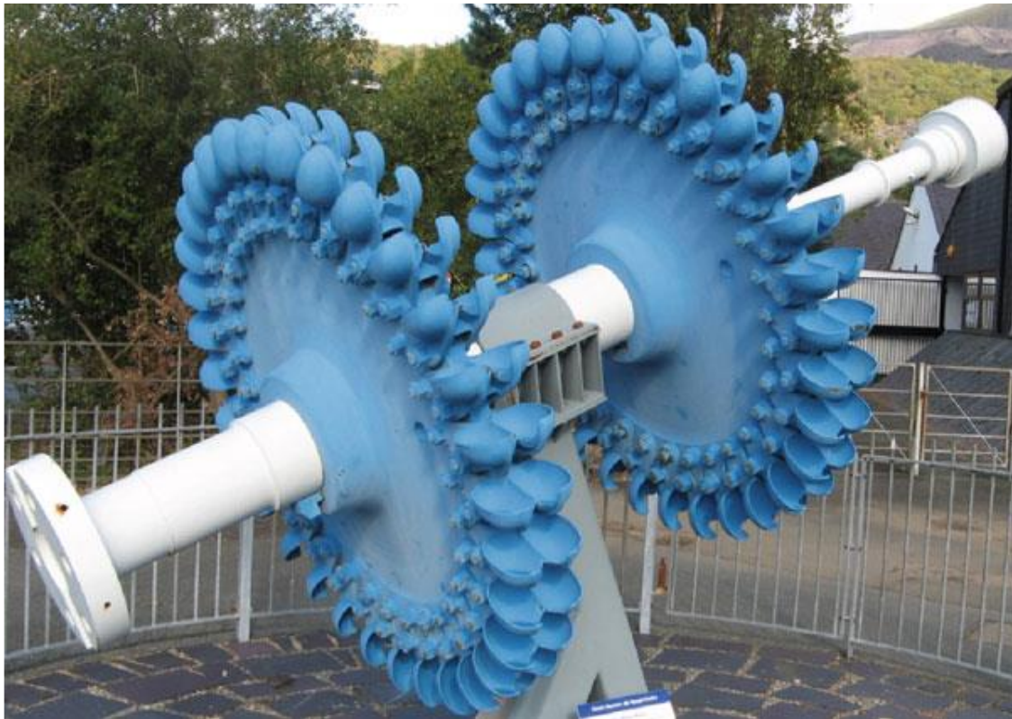
Sl. 2.3. Peltonova turbina (1MW). [1]
