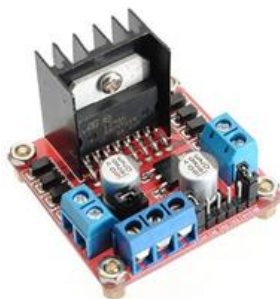
Sl. 3.8. L298N motor driver . [Izvor: http://madrigalelectronics.com/motores-es/stepper-motor-driver/ ]
