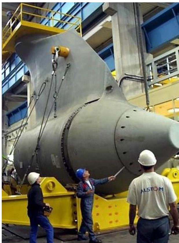
Slika 5.3.5. Azipod propellerski pogon
