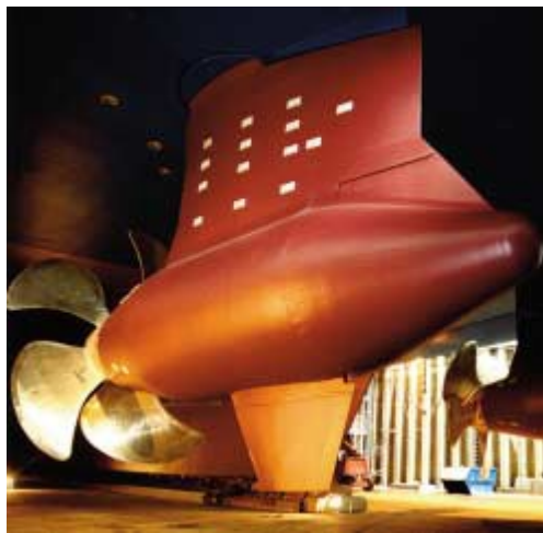
Slika 3.1.3. Radiance of the Seas, 2 x 19,5 MW, Azipod® pogon Izvor: [13]
