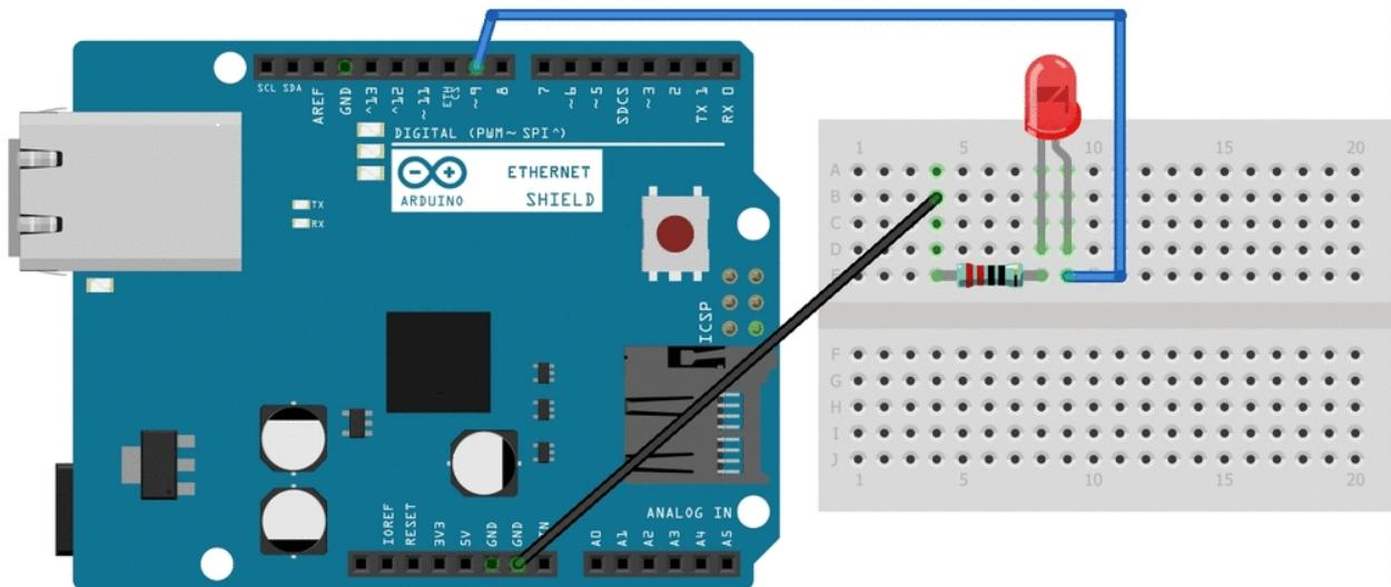
Sl. 3.1. Shema sustava (Arduino Ethernet Shield)
