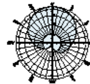
Horizontal pattern ±45°- polarization
