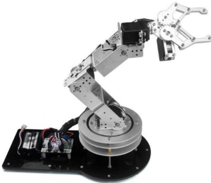
Sl. 2.1.1 Robotski manipulator s bazom.[13]
