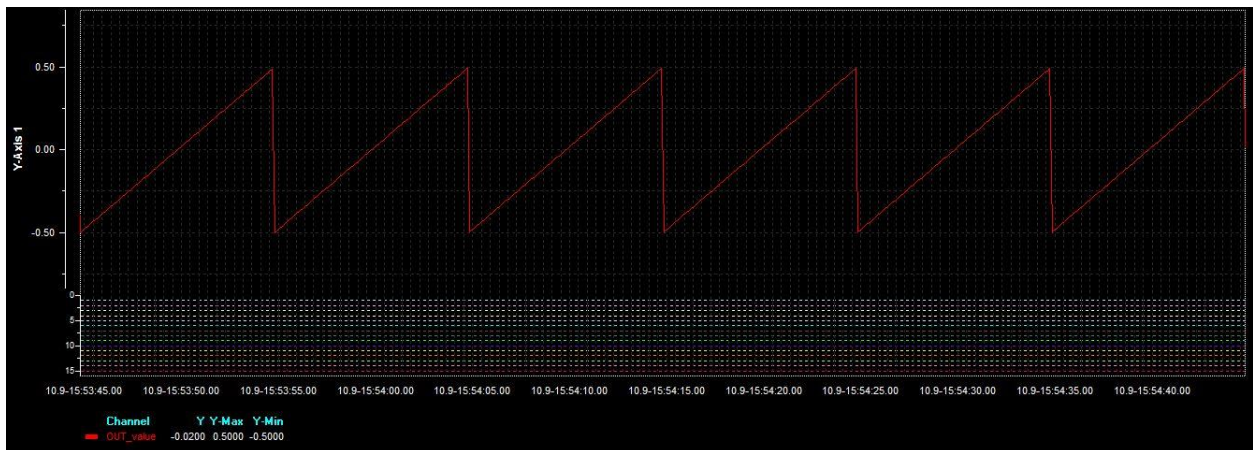
Sl. 4.3. Pilasti signal
