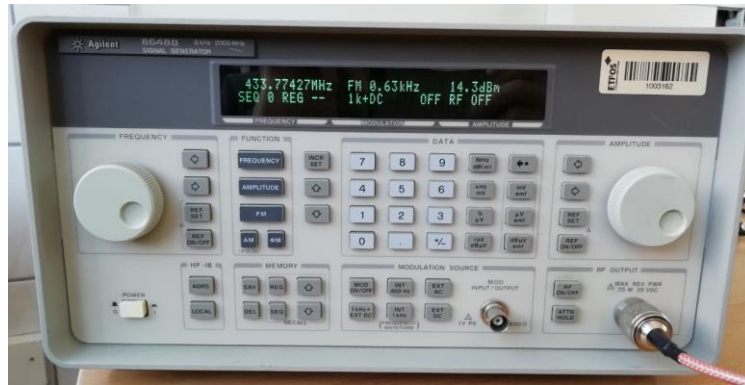
Slika 8.11. Signal generator Agilent 8648B
