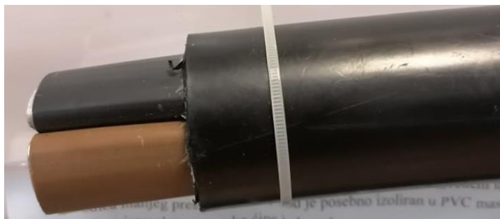
Slika 7.9: Kabel – NAYY-J 4 \times 150 \text{mm}^2
