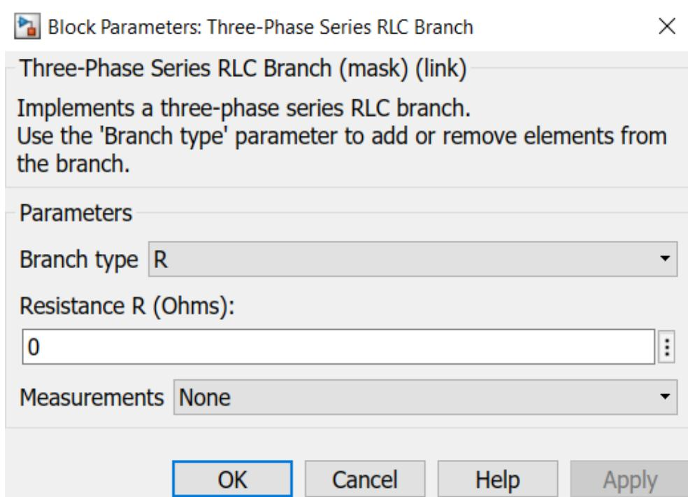
*Slika 5.2. Prikaz parametriranja bloka Three-Phase Series RLC Branch.* [7]
