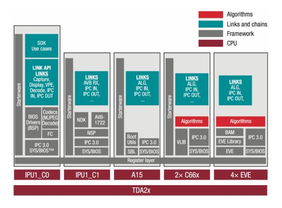
Figure 11: Vision SDK Software Architecture [14]
