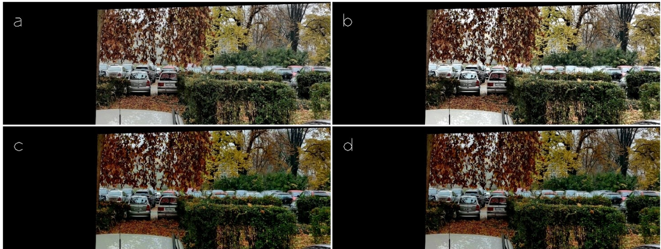
Figure 15: BCE brightness and color equalization for the darker image in figure 12 (a – Brightness equalization using gamma correction, b – Brightness equalization using a basic linear transformation, c – Color equalization using gamma correction, d – Color equalization using basic linear transformation).
