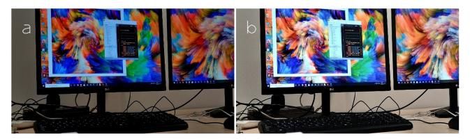
Figure 2: Brightness equalization of the darker image from figure 1 with gain equal to 1.413963 and bias equal to 13.771867 (a – Original image, b – Brightness equalized image using basic linear transformation)
