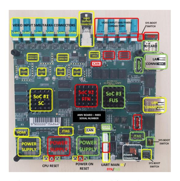
Figure 8: AMV ALPHA ADAS Development Platform Board Layout [12]
