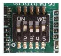
Figure 9: Boot Mode Configuration Switch
