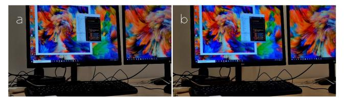
Figure 4: Color equalization of the darker image from figure 1 with gain equal to 1.207584 and bias equal to 3.894011, (a – Original image, b – Color equalized image using basic linear transformation)
