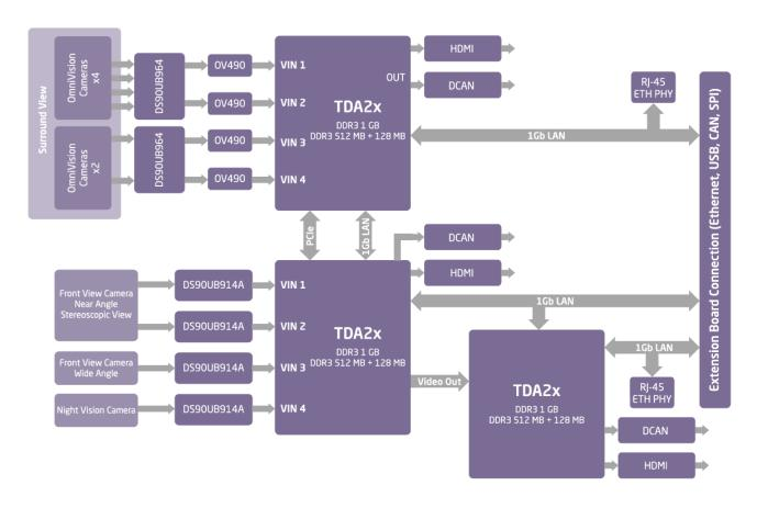
Figure 10: Block Diagram Showing interactions between SoCs [13]
