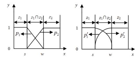
Figure 6: Left - Gradual Fusion Algorithm weight distribution in overlapping region, Right - Improved Gradual Fusion Algorithm weight distribution in the overlapping region. [3]
