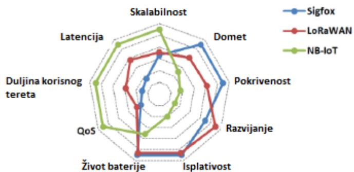
Slika 7.1 Usporedba Sigfox, LoRaWAN i NB-IoT
