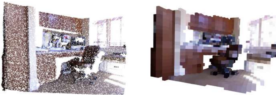
Figure 2.7: An example (Song, Lichtenberg, and Xiao, 2015) of a point cloud (left) with the corresponding voxel grid (right).
