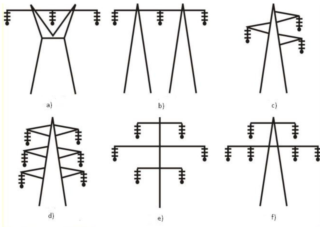
*Slika 6. Najčešće vrste dalekovoda: a) Y stup, b) Portal, c) Jela, d) dvostruka jela, e) Bačva, f)*
