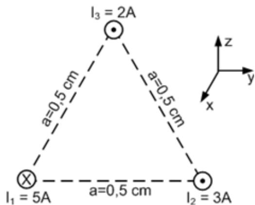
$$I_1 = 5A, \quad I_2 = 3A, \quad I_3 = 2A, \quad a = 0.005, \quad \mu_0 = 4\pi \cdot 10^{-7}$$
