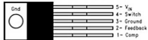
Bent, Staggered Leads 5-Lead TO-220 (T)
