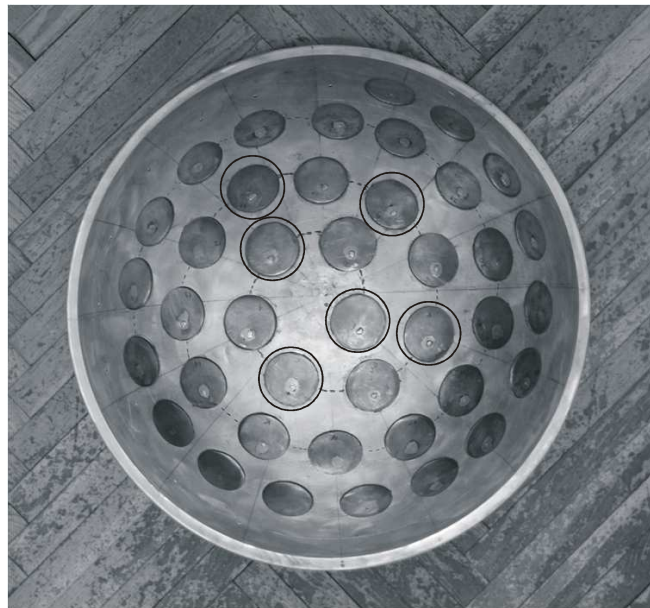
Slika 8.24. Aktivne mikrotrakaste antene sfernog niza spiralnog rasporeda na sferi radijusa 30 cm ( \alpha_1=8,11^\circ , \beta_1=49,94^\circ ; \alpha_2=14,07^\circ , \beta_2=226,18^\circ ; \alpha_3=18,19^\circ , \beta_3=337,99^\circ ; \alpha_4=21,57^\circ , \beta_4=67,22^\circ ; \alpha_5=24,50^\circ , \beta_5=143,93^\circ ; \alpha_6=27,13^\circ , \beta_6=212,40^\circ ).
