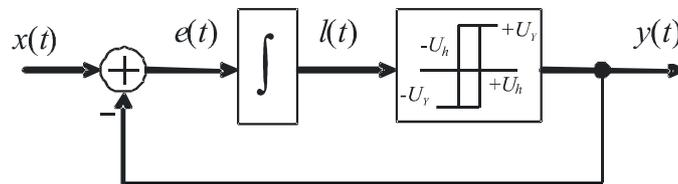
Slika 2.8. Asinkroni sigma-delta modulator
