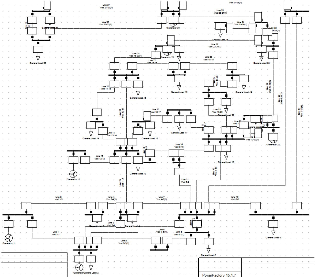
**Slika 4.2.:** Shema IEEE 30 bus System (Test Case) u Power Factory-u
