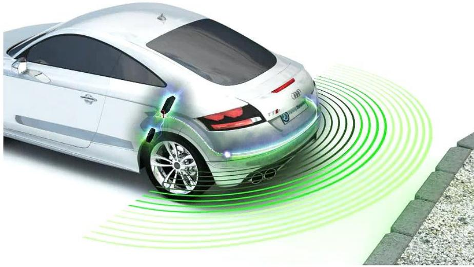
**Slika 2.2. Elektromagnetski sustav parking senzora [5]**
