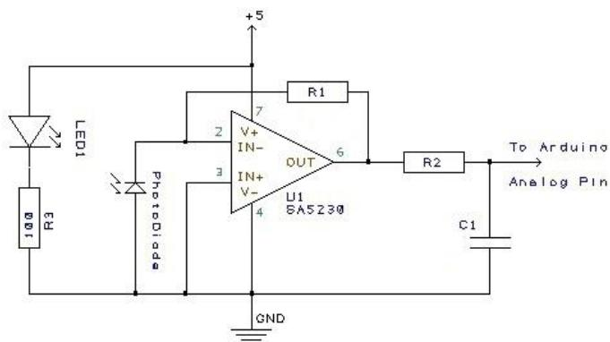
$$\begin{aligned} R1 &= 1M \\ R2 &= 100 \\ C1 &= 4.7 \mu F \end{aligned}$$
