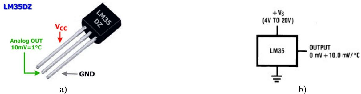
Slika 2.4: a) LM35DZ analogni senzor temperature b) Shema analognog senzora temperature
