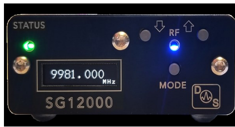
Sl 4.1. Signal generator SG12000 prema [7]
