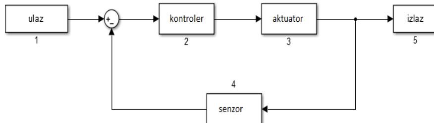
**Slika 2.5** Blok shema regulatora temperature
