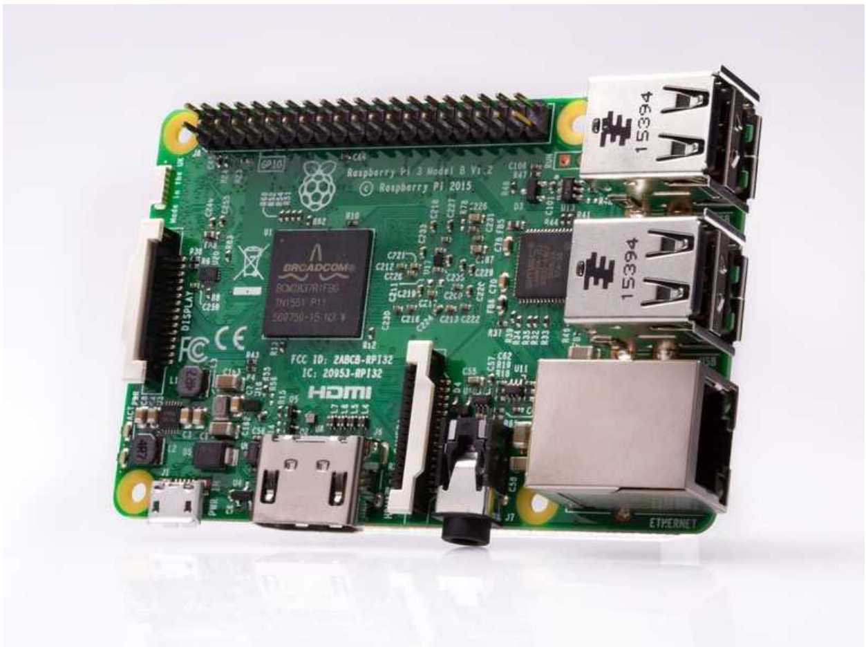
Sl. 2.1 Raspberry Pi 3 model B
