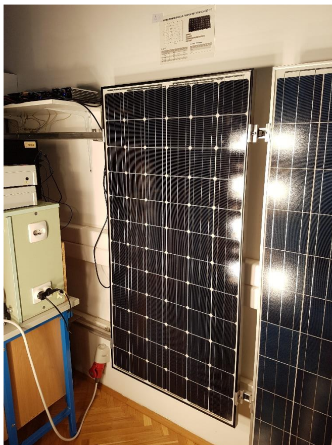
Slika 4.5. FN modul Panasonic VBHN240SE10
