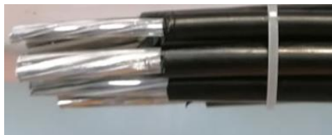
Slika 7.6: Vodić– Elkaleks- 4 \times 70 \text{mm}^2 , 2 \times 16 \text{mm}^2
