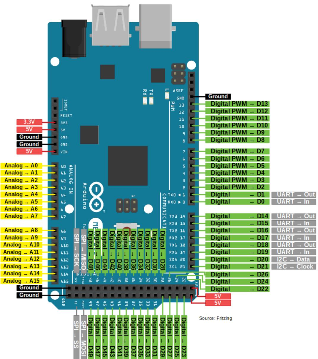
Slika 3.6: Raspored pinova na Arduino MEGA 2560.
