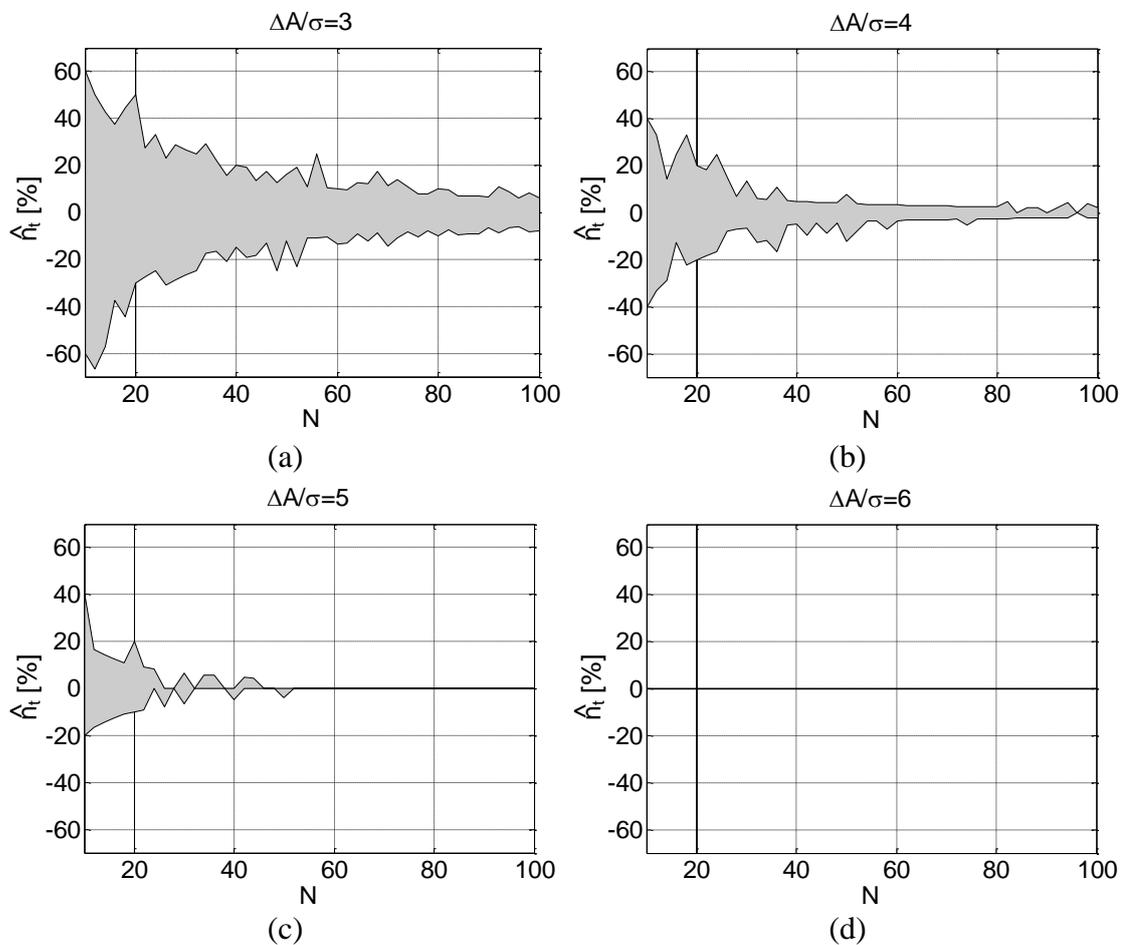
Slika 4.9: Devijacija indeksa SCD metode  $\hat{n}_t$  za  $N \in [10, 100]$ ,  $n_{Gt} = N/2$ ,  $\Delta A = 20$ , (a)  $\Delta A/\sigma = 3$ , (b)  $\Delta A/\sigma = 4$ , (c)  $\Delta A/\sigma = 5$  i (d)  $\Delta A/\sigma = 6$ .
