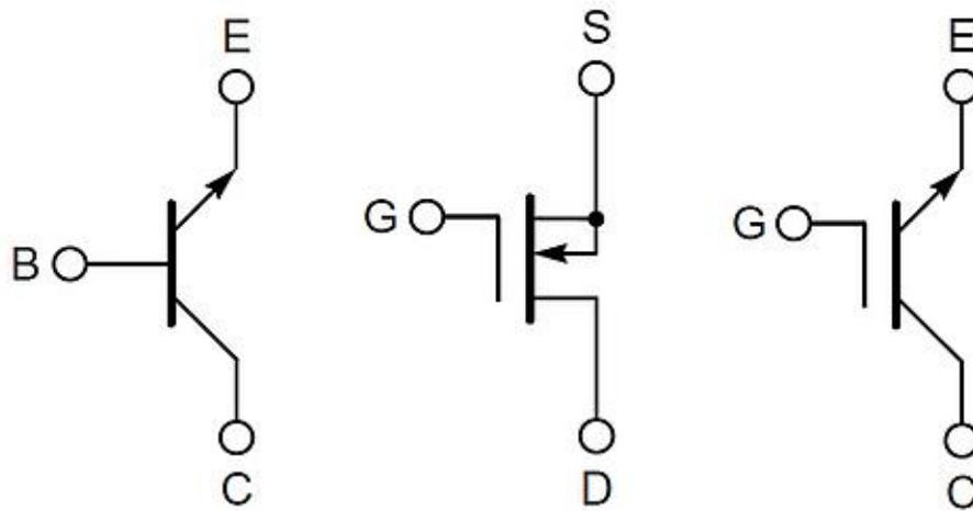
Slika 4.7. Bipolarni tranzistor, MOSFET i IGBT. [19]
