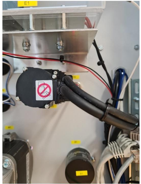
Sl. 2.19 Servomotor HG-KN13J
