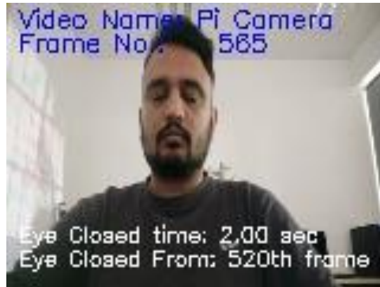
Figure 6.9 Eye long-closed detection (a - Individual close eye at frame 520, b – Arbitrary frame 540 after 0.81 secs, c – Eye long-closed detected after 2 seconds in frame 565)
