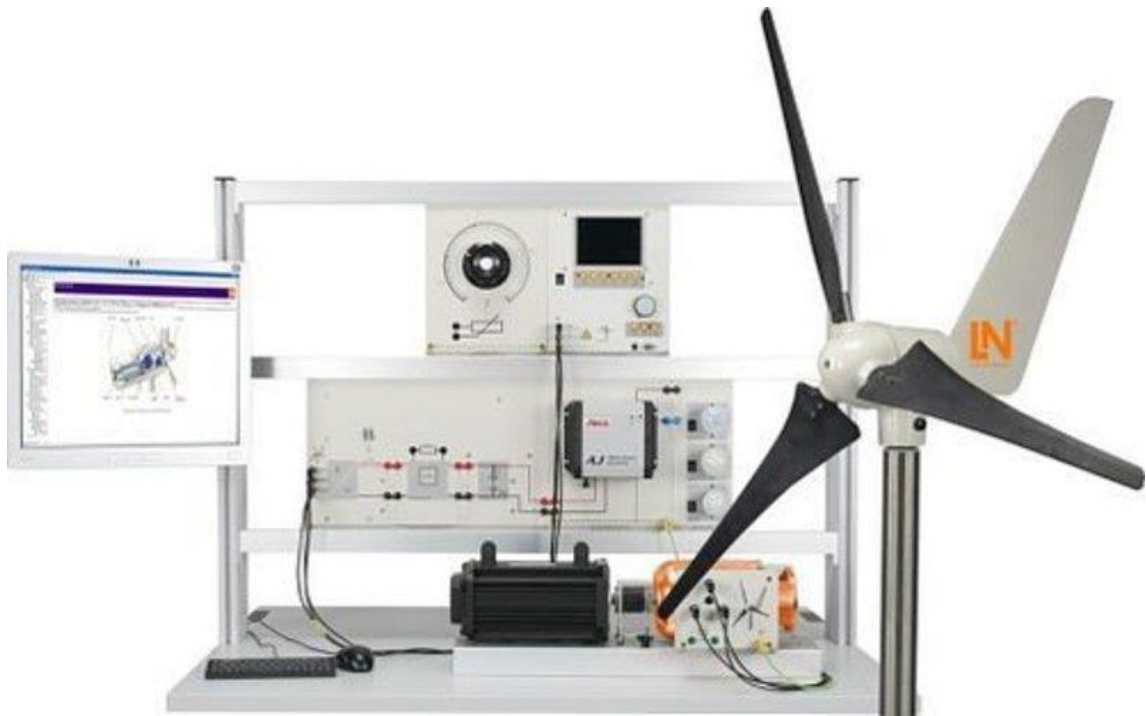
Slika 4.17 EWG 2 Small wind power plant trainer maketa [4]
