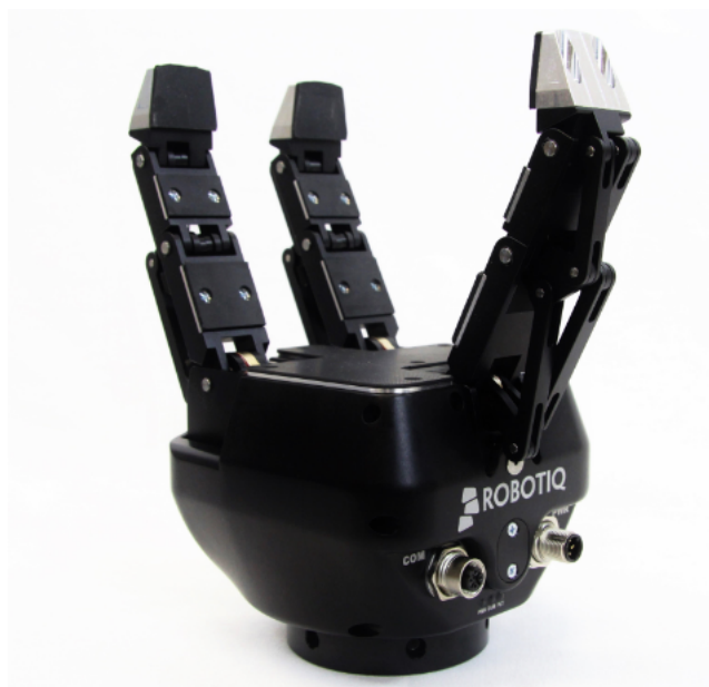
Slika 4.5: Robotiq 3-Finger Gripper. [14]
