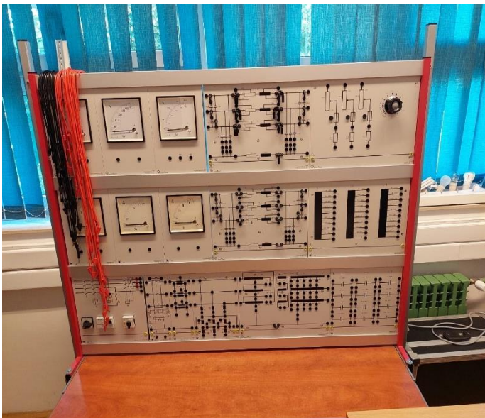
Slika 4.1. Leybold Didactic simulator voda
