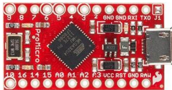
Sl. 3.3. Arduino ProMicro 5V/16MHz
