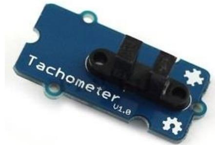
**Sl. 2.8.** Tachometer speed module
