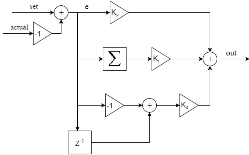
**Shema 4.1.** Shema PID regulatora.
