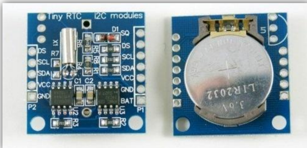
Sl. 2.4. DS1307 Real-time Clock modul
