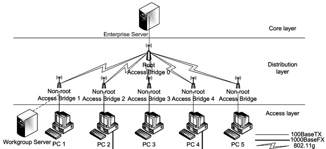
*Figure 2 Structure of experimental MAN
