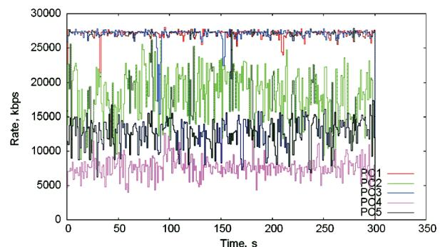
**Figure 5** PC1 to PC5 throughput in the point-to-point mode
