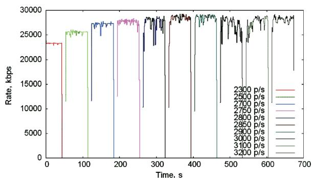
*Figure 3 Link throughput in relation to the number of packets
