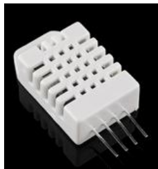
Sl. 3.12. Senzor vlažnosti i temperature DHT22 (RHT03). [Izvor: https://www.sparkfun.com/products/10167 ]
