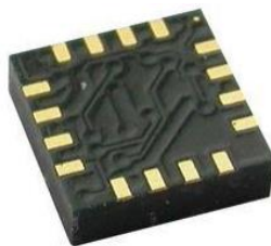
Sl. 3.16. Magnetometar HMC5883L. [Izvor: https://www.sparkfun.com ]
