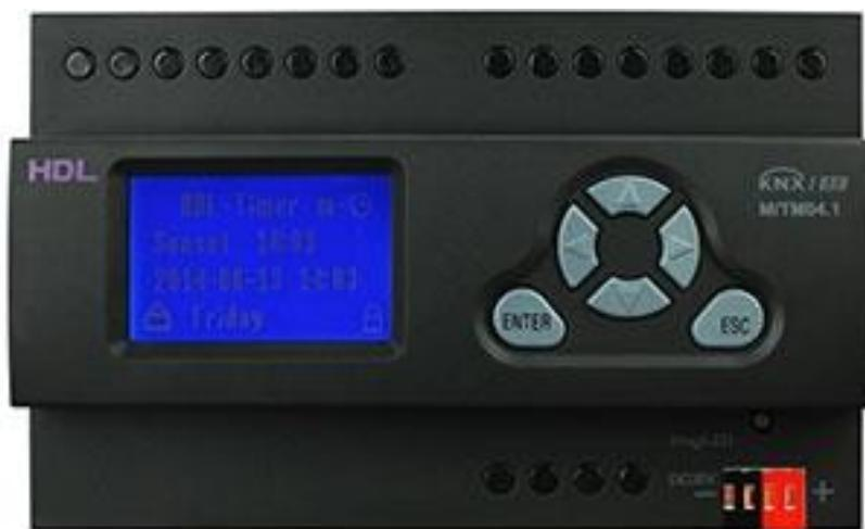
Slika 4.3. Vremenski aktuator(Timer Actuator 4CH Master-Slave) [27]
