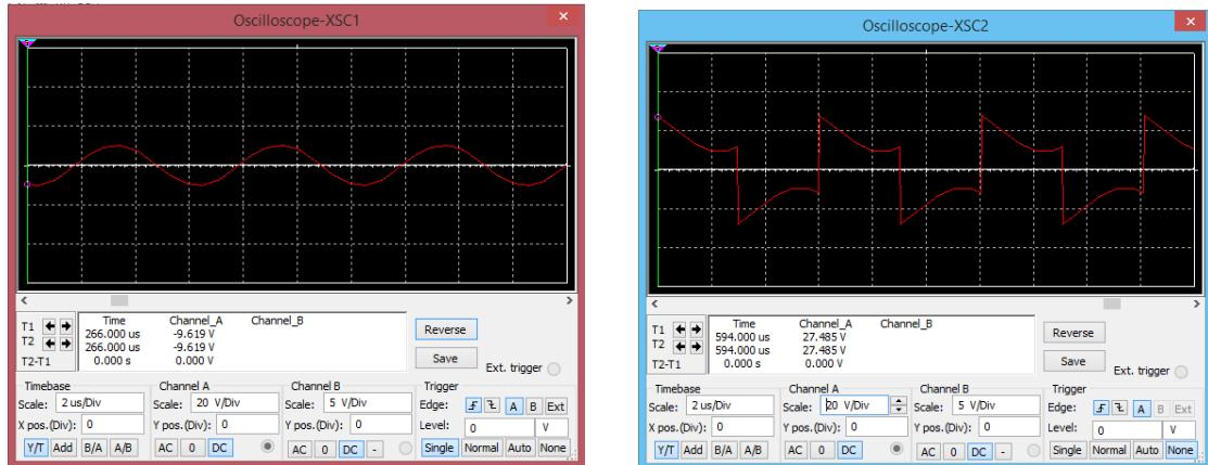
*Sl. 3.10. Paralelni LC krug ( $L = 233 \mu\text{H}$ )*
