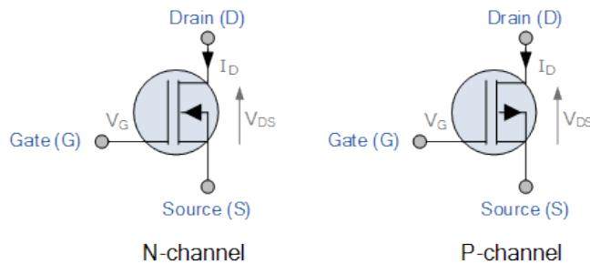
**Slika 3.19:** Shematski simbol MOSFET
