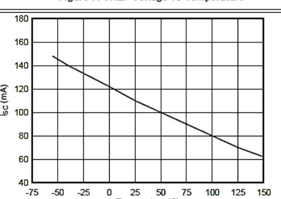
Figure 5. VREF Short-Circuit Current vs Temperature for  $V_{CC} = 15\text{ V}$
