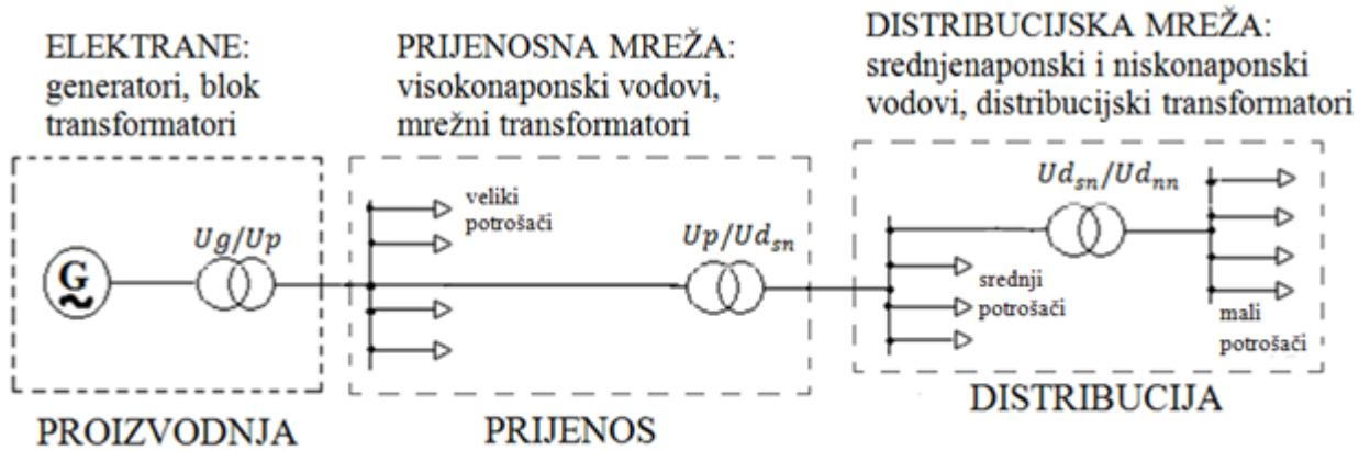
$Ug$  = Napon generatora (4 kV, 12 kV, 16 kV, 25 kV, itd.)
