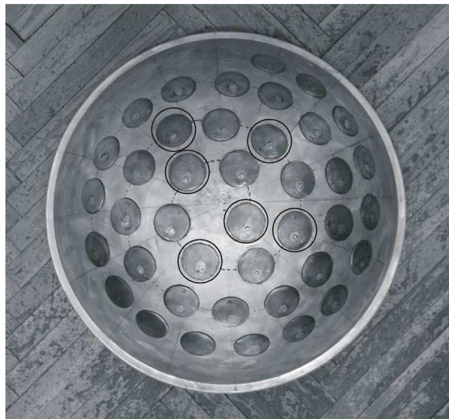
**Slika 8.24.** Aktivne mikrotraktaste antene sfernog niza spiralnog rasporeda na sferi radijusa 30 cm ( $\alpha_1=8,11^\circ, \beta_1=49,94^\circ; \alpha_2=14,07^\circ, \beta_2=226,18^\circ; \alpha_3=18,19^\circ, \beta_3=337,99^\circ; \alpha_4=21,57^\circ, \beta_4=67,22^\circ; \alpha_5=24,50^\circ, \beta_5=143,93^\circ; \alpha_6=27,13^\circ, \beta_6=212,40^\circ$ ).
