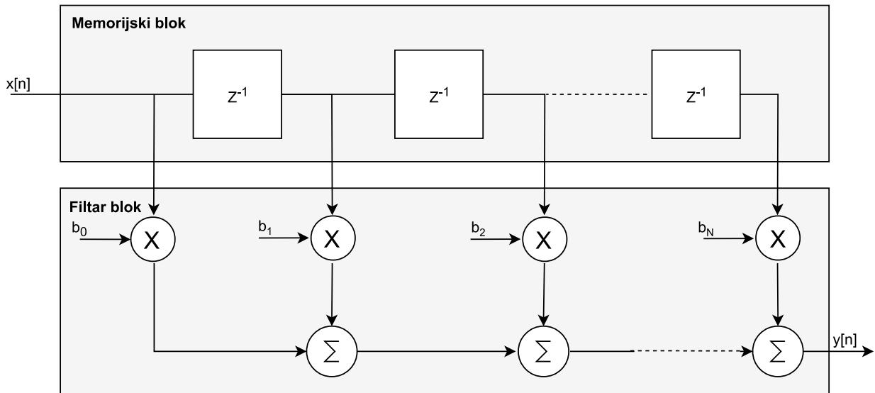
Sl. 4.2 Blok shema FIR filtra unutar FPGA
