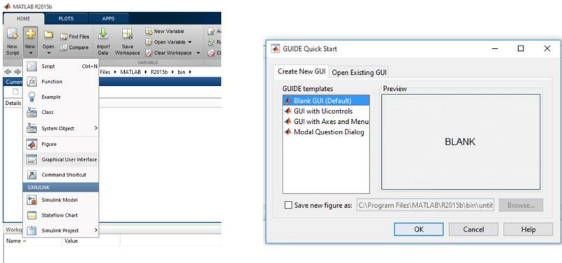
**Sl. 4.1.** Home → New → Graphical User Interface → Create New GUI → Blank GUI
